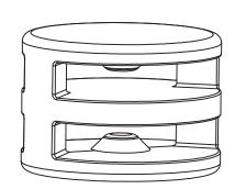
MUST BE FREE OF BURR, CRACK, SHRINKAGE AND IMPERFECTIONS THAT AFFECY FUNCTION TEMPERATURE RANGE: -  $40^{\circ}$ C ~+  $120^{\circ}$ C UNFILLED DIMENSIONS AS SHOWN IN 3D
