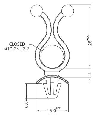
MOUNTING HOLE Ø6 CHASSIS THICKNESS 0.78~2.0mm
