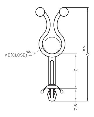
HOLE IN CHASSIS Ø4.8 CHASSIS THICKNESS 0.8~2.2
