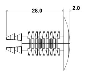
MOUTING HOLE: Ø 6,9 THICKNESS: 1,0 - 20,0
