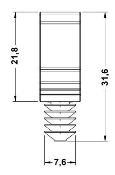
MOUNTING HOLE Ø7,0 THICKNESS 0,9 - 2,6
