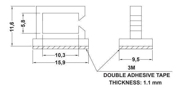
NOTE: 1. THE HEIGHT IS NOT INCLUDE THE RELEASING PAPER AND ADHESIVE TAPE'S THICKNESS.
