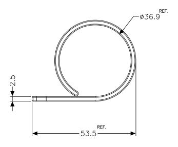
NOTE:1.All measurement does not include gate which raises under 0.3mm. 2.It is normal if it is shrinking.
