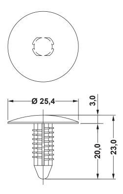
MOUNTING HOLE: Ø7.0mm PANEL THICKNESS: 2.54~20mm
