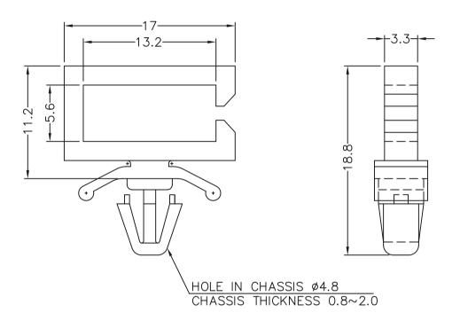
NOTE: All measurement does not include gate which raises under 0.3mm.
