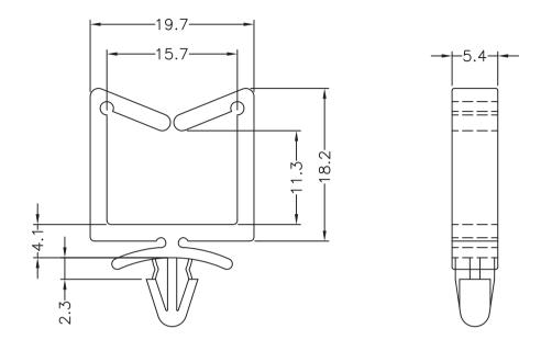
HOLE IN CHASSIS Ø4.8~Ø5.0 CHASSIS THICKNESS 1.2~2.1
