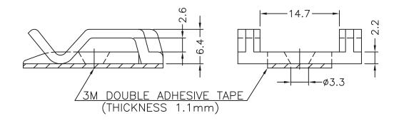
NOTE:1. The Height is not include the releasing paper and adhesive tape's thickness.
