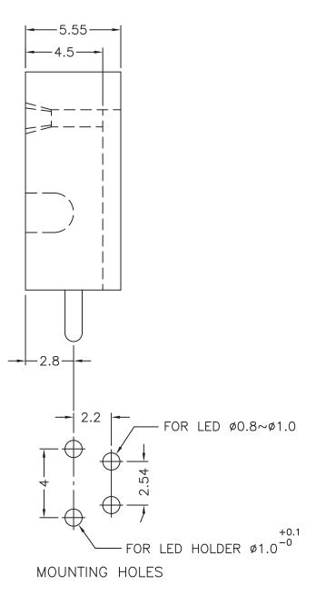
NOTE: All measurement does not include gate which raises under 0.3mm.
