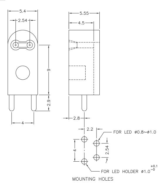
NOTE: All measurement does not include gate which raises under 0.3mm.
