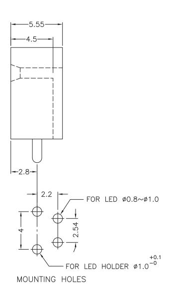
NOTE: All measurement does not include gate which raises under 0.3mm.
