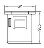
A: HOLE IN CHASSIS: Ø7.5 CHASSIS THICKNESS: 1.0~1.5mm
