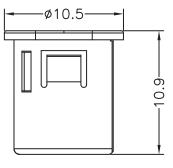
A: HOLE IN CHASSIS: \$\phi 9.0^{\frac{+0.05}{0.05}}\$
