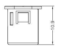
HOLE IN CHASSIS: Ø9.0 CHASSIS THICKNESS: 0.6~1.0
