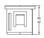
A: HOLE IN CHASSIS: Ø6.35~Ø6.4 CHASSIS THICKNESS: 1.0~1.2
