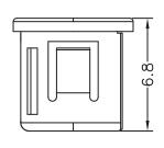
A: HOLE IN CHASSIS: Ø6.35~Ø6.4 CHASSIS THICKNESS: 0.8~1.0
