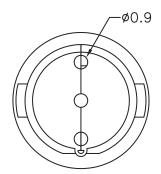
NOTE:1.All measurement does not include gate which raises under 0.3mm. 2.Suitable for  $\emptyset$ 3 LED with visor and 3PIN.
