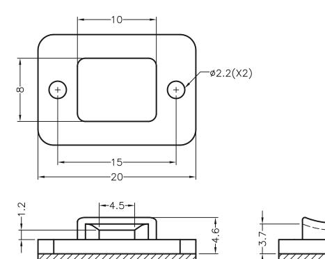
3M DOUBLE ADHESIVE TAPE (THICKNESS 0.9mm)
